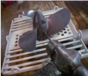
Once the shaft is clean slide the new propeller on, line up the pin hole and tap the roll pin completely into place. Once the roll pin is in place re-install the propeller cage.
