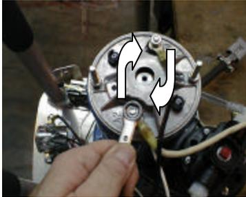
With the Pacific Motors (Light blue in color) the direction can be changed by removing the motor cap and switching the power and ground leads . Re- install motor cap and you are done.
