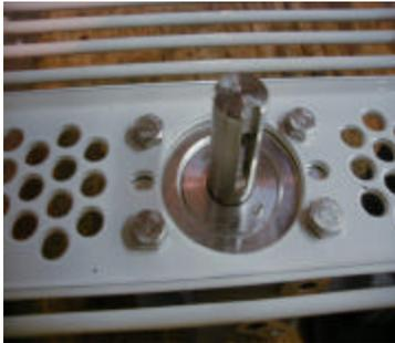
Once the propeller is removed, it is very important to clean the gearbox shaft. It can be sanded lightly with a fine grade sand paper it help remove any corrosion. It must be completely clean prior to attempting to install the new propeller.
