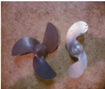
The 3 blade propeller is designed to turn in the opposite direction than the 2 blade propeller. The next step will be to change the direction the motor turns.
