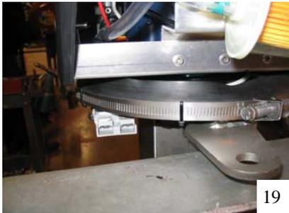
Install the rubber strip around the UHMW plate. Tighten the hose clamp around the rubber strip. The two zip ties are provided to keep the excess clamp tucked in neatly. (fig. 19)
