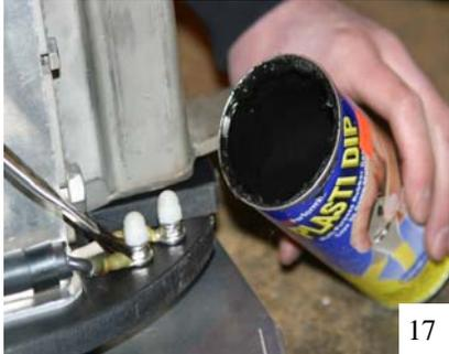
Finish by installing the nylon acorn nuts. Apply plastic dip to the terminal in an effort to help stop corrosion. (fig. 17) Connect all leads to corresponding post taking not on which is positive and negative. Visually inspect the flex wire as you rotate unit from side to side to insure that no binding occurs. (fig. 18)
