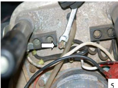
In order to remove the slip rings you must first remove all the brass nuts on the back side. (fig. 5) Now remove all the bolts and slip rings. These items are no longer used in the update. (fig. 6)
