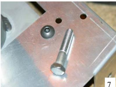
Be sure to replace the four 3/8 hex headed bolts with the supplied allen cap headed bolts. (fig. 7) It is crucial that you make sure that the nylon sleeve is still located in mount. Next mount the flex wire to the mount plate. It is important to install the lead in this order: 1.plastic shoulder washer (shoulder facing down) 2.terminal 3. supplied brass phillips screw (fig. 8)
