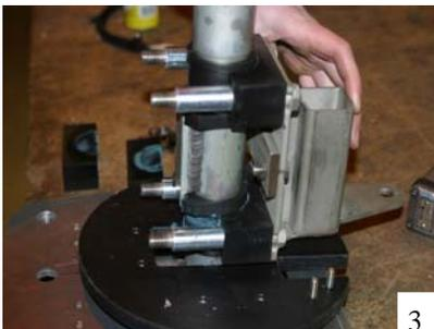
With all hardware loose remove the pivot assembly. (fig. 3) Lift the mount plate so that you can access the slip rings. (fig. 4)
