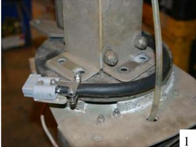
Begin by removing the SB-50 connector and cable assembly.(fig.1)
