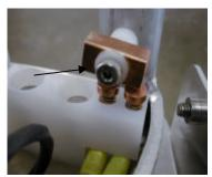
Remove both of the contact bars, save the bolt and the nylon bushings. One of the three bushings will be re-used along with the bolt.
