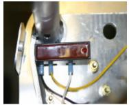
Install solid state switches through the same holes the contact block was mounted through. Re-used the nuts that held the contact block to the handle bar plate.
