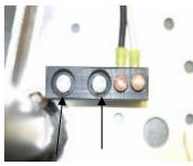
Remove both of the contact block assemblies, including the wires by removing the two bolts that hold the contact block to the handle bar plate. You will need to hold the nuts on the bottom of the plate, be sure to save the nuts as they will be reused. Leave the wires attached to the to the contact block assembly, the new solid state switches have new wires pre-attached.
