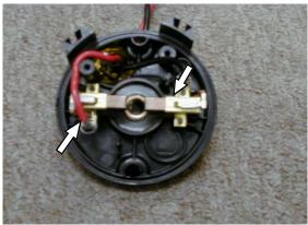
• Clean the Brush and cap assembly with electric motor cleaner.
