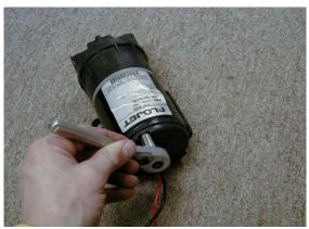
• Reinstall and tighten end cap bolts.
