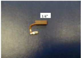
Measure both Brushes length if either is 1/4 of an inch or less both Brushes should be replaced.
