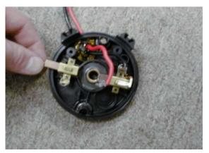
• With the Brushes removed clean the entire assembly with an electrical motor cleaner.
