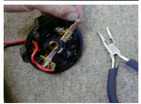
Re-install Brushes and connect wire to terminal on Brush holder, lightly spray brushes with \*Corrosion Block.
