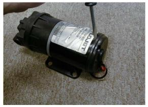
• Using a small flat head screw driver between the end cap and the motor case lightly pry end cap off the motor case.
