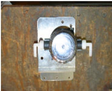
Install the 90 degree barbed fittings in the screen filter. Using the 8/32 x 3/8 machine screws, install the screen filter on the squirt pump bracket. The arrow must be at the top facing the right.
