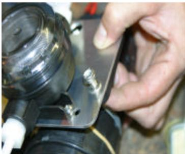
Using the 1/4 button head Allen bolts install the squirt pump on the opposite side of the squirt pump from the screen filter. Be sure on both sides of the Allen bolt, use a 1/4 washer as shown on the right.
