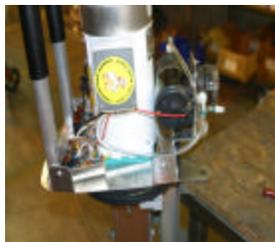
The red wire from the squirt pump is routed along side of the motor and connects to the terminal shown on the right. Tighten the brass screw to snug.
