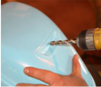
Using a 5/16 drill bit, drill a hole in the center of the notched area of the motor hood.
