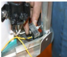
Install the magnetic trigger, be sure that the magnet is on the lower side closest to the solid state switch. Install the motor cover. Be sure to plug the squirt hose to the motor cover.
