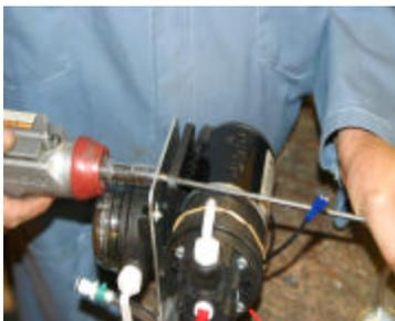
Tighten the squirt pump to the squirt pump bracket. Rivet the bracket to the motor cover plate then follow the hose diagram on the next page.
