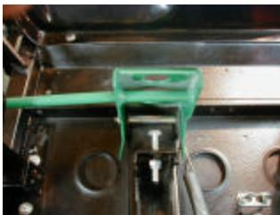
4. When all adjustments are complete, double check all jam nuts to be sure they are tight. Blue locktite can be used to be sure jam nuts will not move.
