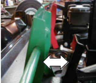
1. Begin by setting the speed on your Kart, all speed adjustments should begin by the pedal stop located behind the gas pedal. By screwing the bolt inward you will make the Kart faster, by screwing the bolt outward it will slow the Kart down.
