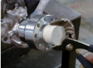
1. Begin by removing the dust cap, using Channel Locks grasp the dust cap firmly and work up and down while pulling outward as well. Remove the cotter pin and castle nut set aside the castle nut and dust cap. Throw away the cotter pin, it will not be re-used.
