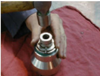
4. Install rear Wheel Bearing and rear Wheel Bearing Seal. Use a large seal installation tool to avoid damaging seal.
