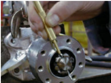
7. Install a new cotter pin, using a brass drift punch, tap the head of the cotter pin down into the castle nut. When complete the head of the cotter pin should be crushed just slightly.
