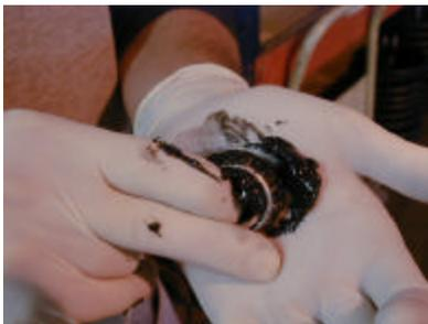
3. Pack Wheel Bearings with Wheel Bearing Grease either by hand or with Wheel Bearing packing tool, forcing grease into the cage and roller assembly. Put a film of grease on the Both Wheel Bearing Races and on the Spindle shaft.
