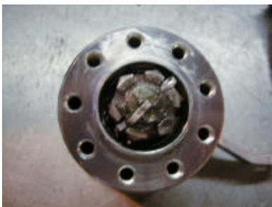
Fold the front half of the cotter pin over the Spindle and cut of the back half with a pair of cutter (as seen in the picture) Re-install the dust cover.
