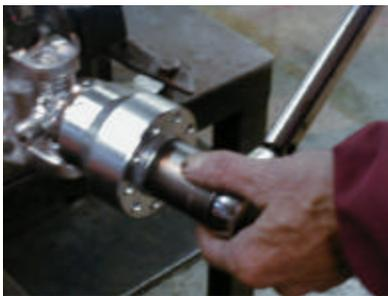
6. Install the front Wheel Bearing and castle nut, torque the castle nut to 15 ft. lbs to seat the Wheel Bearings properly. Then loosen the castle nut to finger tight and rotate the Hub Assembly the hub should rotate freely. Line up the hole for the cotter pin through the castle nut by tightening the castle nut then double check that the Hub Assembly rotates freely and has no play on the Spindle.
