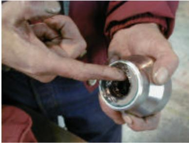
5. Put a light film of grease around the lip of the Grease Seal to keep it from tearing during installation. Wipe of the excess grease prior to installing.
