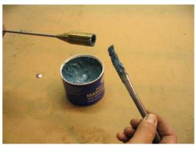
• Before installing new shaft coat both ends with marine grease. Applying grease will help reduce corrosion.
