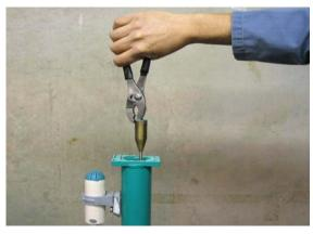
• With pliers grasp the end of the shaft and remove.
